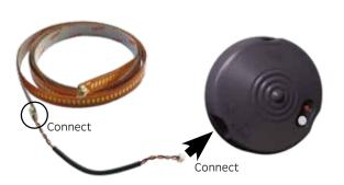
The moisture sensor strip can be joined for longer moisture detection zones, but should not be longer than 2 lengths / 6 metres.
