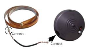
The moisture sensor strip can be joined for longer moisture detection zones, but should not be longer than 6 lengths / 6 metres.
